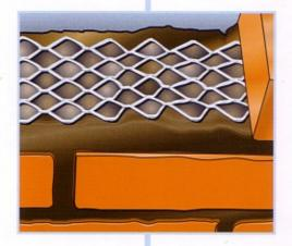
DYNTEK CoilMesh is used for the reinforcement of brickworks and blockworks by embedding in mortar joint between courses of bricks or blocks. It can also be used as plaster reinforcement over conduits and services.
