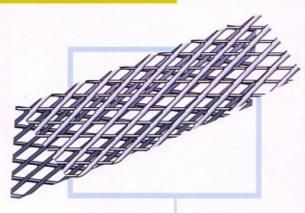
DYNTEK CornerMesh is used at inward facing corner to prevent and resist crack/s due to differential thermal movement/s. Tensions become particularly strong at inward facing corners where movements can come from opposing directions. Hence DYNTEK CornerMesh is made heavier and stronger than the average StripMesh.
